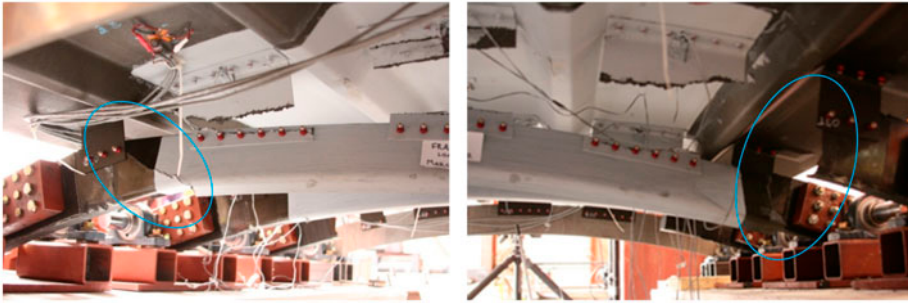
Figure 14. Dynamic specimen Frame03 fracture of frames near boundary supports.
